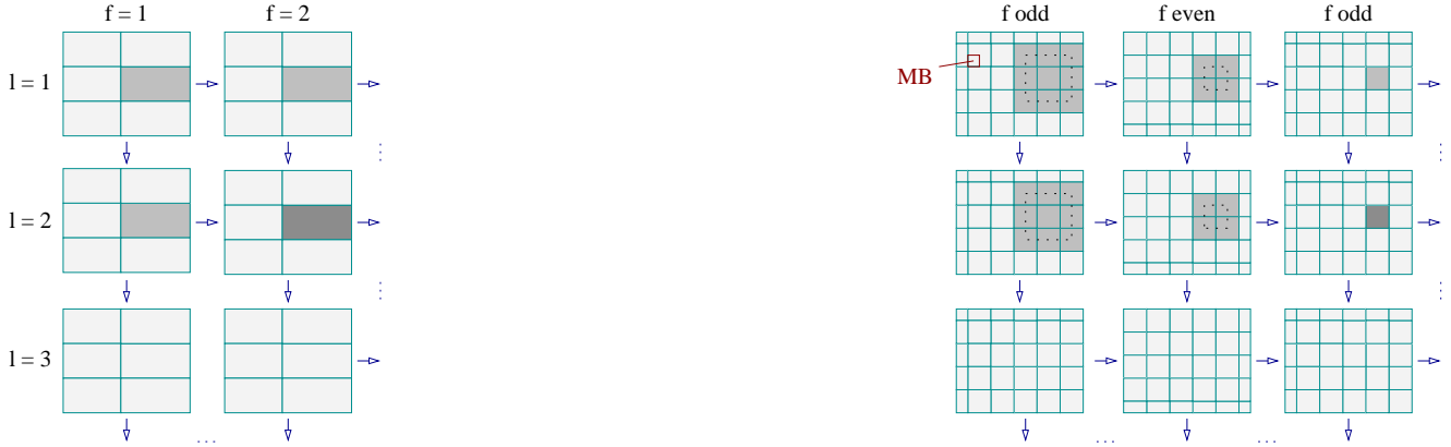
Figure 2: The dark-gray shaded segments are recursively predicted from the light-gray shaded segments. Left: Scenario A with F = 2 , L = 3 , X = 2 , Y = 3 . Right: Scenario B with F = 3 , L = 3 , X = 6 , Y = 5 . Both scenarios are examples for segment structuring of the QCIF image format.
