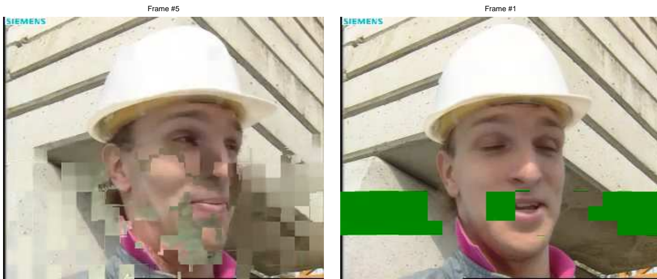
(a) Spatial and temporal concealment coupled with random constrained INTRA updates. 2 slices per picture. Fourth frame after error occurrence
