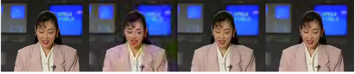
Figure 4: Original (left) and decoded frame 100 of AKIYO. Middle left: Dirac; Middle right: Theora; Right: H.264. The images may be slightly scaled due to space considerations
